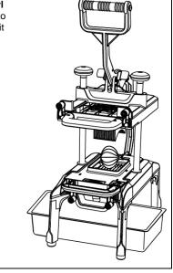
Pull the handle on the chassis down. Place one hand on the handle and the other hand on the palm rest. Lift the handle up, then use your thumb to open the handle latch and then pull the handle swiftly down.
