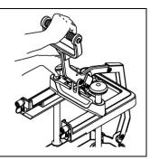
Move the cartridge locking pins to the unlocked position. Move each of the two upper cartridge locking pins and the two lower cartridge locking pins to a horizontal position so the cartridge can be inserted.
