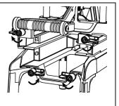
Holding the pusher and blade components together as one cartridge, insert into the chassis. With the pusher component facing up (solid face), guide the sides of the pusher component into the C-shaped channel in the chassis. The blade component will automatically be correctly inserted.
