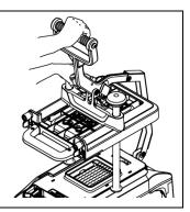
2 Ensure the cartridge locking pins are in the locked (vertical) position.
