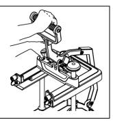
Move the cartridge locking pins to the unlocked position.
