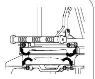
Holding the pusher and blade components together as one cartridge, remove from the chassis. Guide the sides of the pusher component out of the C-shaped channel in the chassis.
