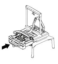
Move the cartridge locking pins to the locked position.
