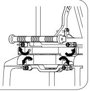
Holding the pusher and blade components together as one cartridge, insert into the chassis. With the pusher component facing up (solid face), guide the sides of the pusher component into the C-shaped channel in the chassis. The blade component will automatically be correctly inserted.
