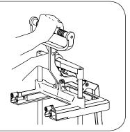
Move the cartridge locking pins to the unlocked position. Move the two upper cartridge locking pins and the two lower cartridge locking pins to their horizontal positions so the cartridge can
