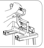
Move the cartridge locking pins to the unlocked position. Move the two upper cartridge locking pins and the two lower cartridge locking pins to their horizontal positions
